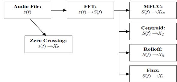
Figure 3. Dataflow Diagram for Timbre Features
